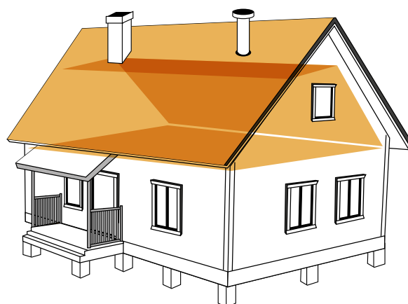
Figure 52. Plywood in attic renovations
